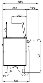
D = Drain El = Electrical inlet (power)
